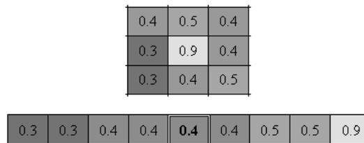
Figure 1: Filtering 3x3 portion of the depth map
